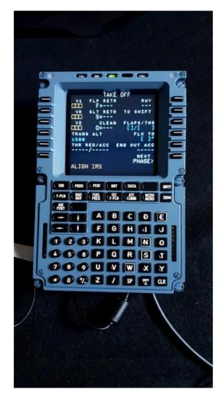
The MCDU is equipped with a Plug'n'Play Ethernet motherboard for XPLANE 11 and Flight Factor A320 Ultimate or PROSIM A322.
